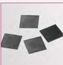
Synthetic Diamond: Slicing of CVD diamonds
